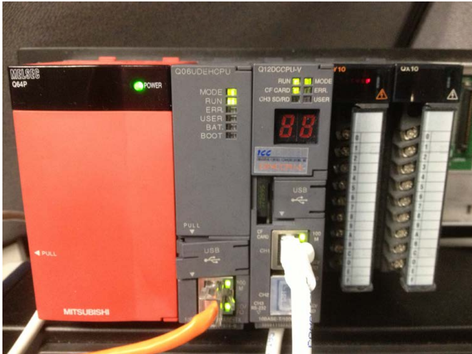
Figure 1 Q38DB Rack with an iQCPU and an EIP4CCPU Master Module Installed
